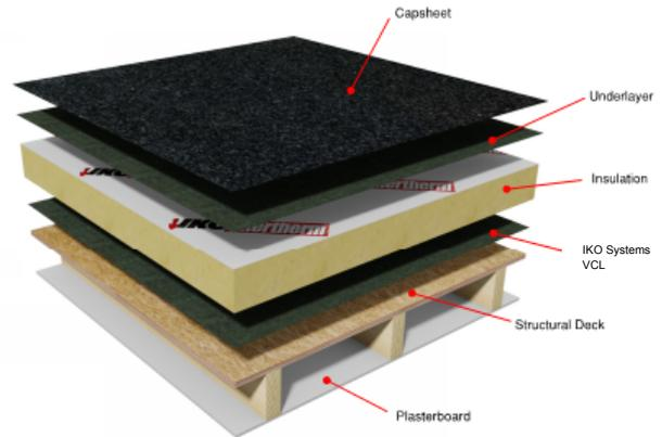
Figure 1 – Typical Warm roof build up (BUR).
